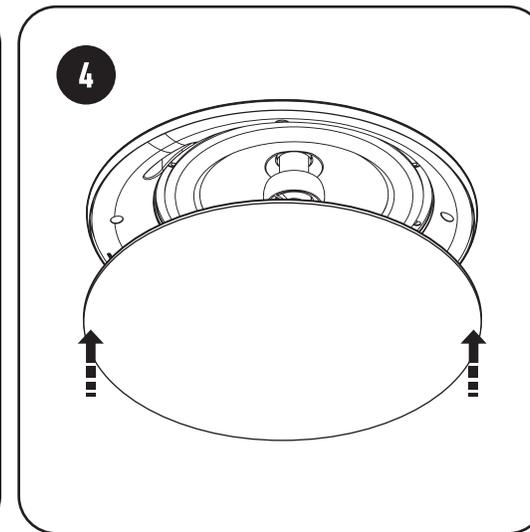
⚠️ **MAX 5Kgf/cm (4.34 lbf/inch.) or 0.5 NM when tightening the dog leg screws.**
